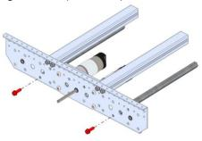
**Step 20:** Attach four 63mm Churro Extrusions (am-3399) to one of the Inside Plates using 1/4-20 Self-Tapping Screws (am-1310) in the positions indicated in the diagram.
