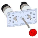
**Step 9:** Ensure that all of the gears are aligned with each other and tighten the #10-32 Set screws to lock all the gear assemblies in place.
